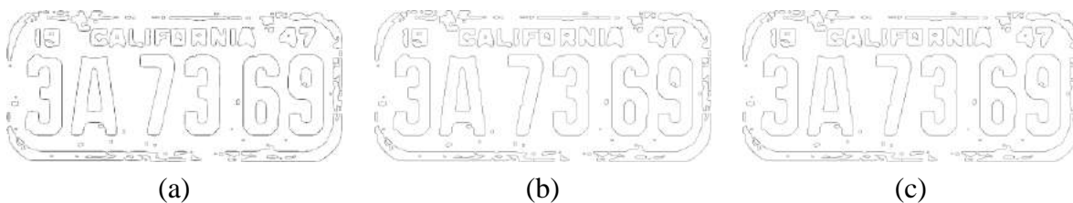
Figure 10. Edges detected by the proposed (a) hybrid-Canny, (b) hybrid-Sobel, and (c) hybrid-Prewitt edge detection methods on the test image.
