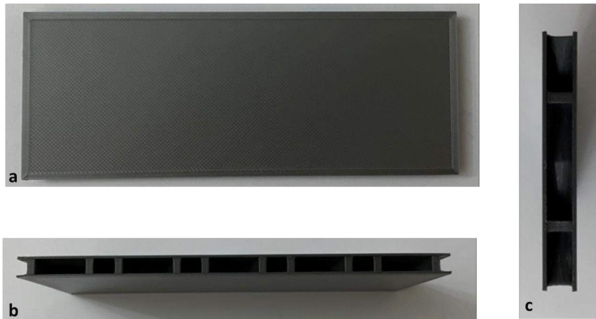
Figure 2.5: Sandwich Panel After Adhesion; a) Front view, b) Top view c) Side view
